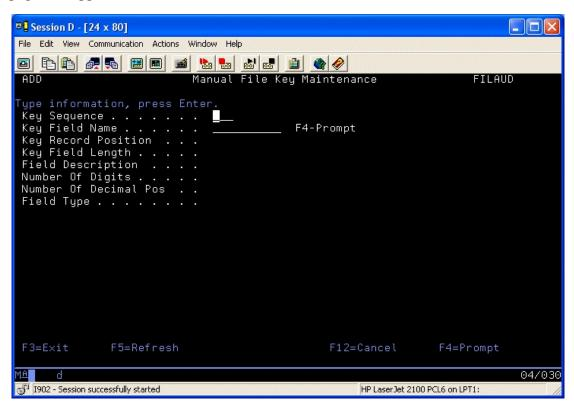
The key sequence field controls the position of the field within the key. Assign these values sequentially starting with the number one. To choose field names, position the cursor in the Key Field name and press the F4 key. A field selection window will appear as follows:
