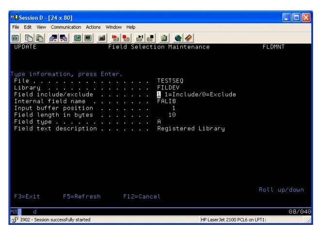
The only field that you will have access to is the Field Include/Exclude field. Leaving the value set to '1' will include the field in the iFileAudit analysis process. Changing the value to '0' will exclude the field from all iFileAudit processing.
