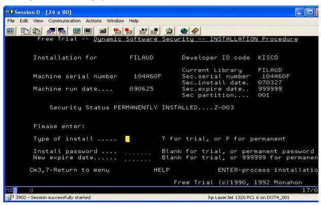
The message at the center of the screen indicates your current installation status. You should also check the Sec. expire date for an expired trial period. iFileAudit may still show as installed on a trial basis but, if the trial is expired, it will no longer function.
