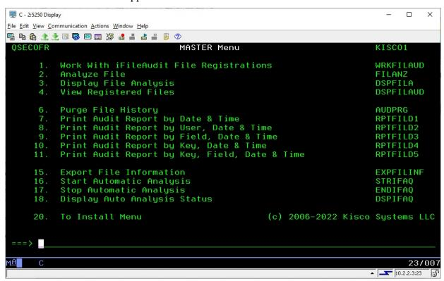
Each menu option handles the following functions. The right margin of the menu display shows the command that is run by that option. All commands are located in the application library named FILAUD. Each function is described in more detail later in this manual:
