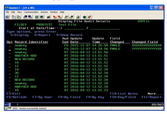
This display will show you all of the file changes that have been made to this file in chronological order. If there is a manual note associated with the change, the Changed Field will display in red. For details about a specific change, place a 5 next to the line in question and press ENTER. A detail screen will be displayed. You can also use option 6 on any line to start a report prompt using the values for the record displayed.
