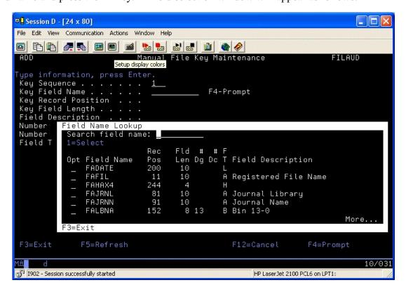
If your non-keyed file has associated logical files that contain key structures, you can ask iFileAudit to locate and list all of these logical files by using the F4=Show Alt Views functions from the initial key maintenance screen. To use one of these key structures, just select the one you want from the list and iFileAudit will automatically adapt to that key structure.
