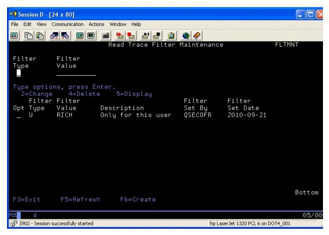
When file read activity is traced, keep in mind that all of the individual fields will not be captured by iFileAudit, just the record key for the file. Because of this, it is important that any non-keyed files have a key structure specified for them to make record identification easier.
